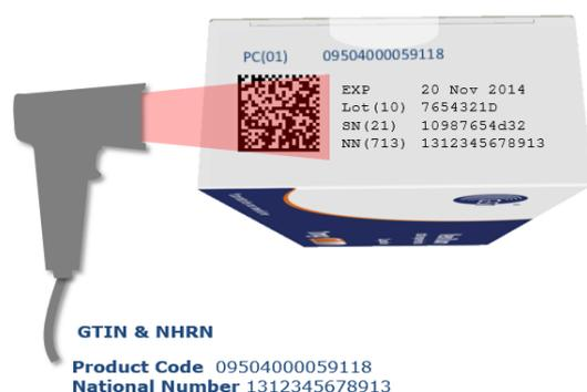
Figure 3 - GTIN coded pack with included NHRN
